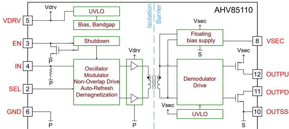
Figure 1: AHV85110 Block Diagram
