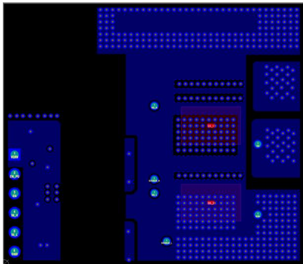
Figure 16: PCB Bottom Layer
