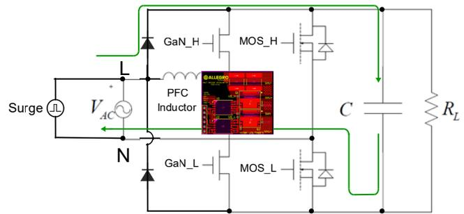
Figure 6: Example of unwanted magnetic coupling due to poor routing of high-current loop under the isolated gate drivers
