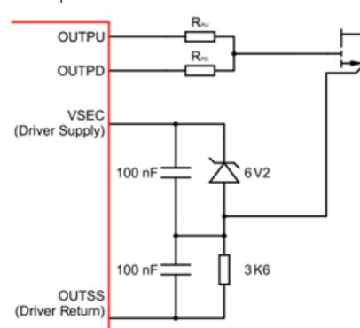
Figure 3: Bipolar output drive schematic
