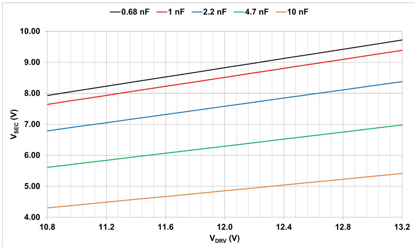
Figure 4: Typical V<sub>SEC</sub> versus V<sub>DRV</sub> for five C<sub>OUT</sub> capacitors; Conditions: f<sub>IN</sub> = 100 kHz, D = 50%, C<sub>SEC</sub> = 20 × C<sub>OUT</sub>
