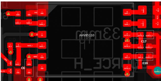
Figure 11: Decoupling capacitor placement
