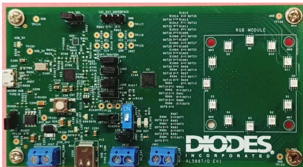
Figure 1. Image of AL5887 Demo Board
