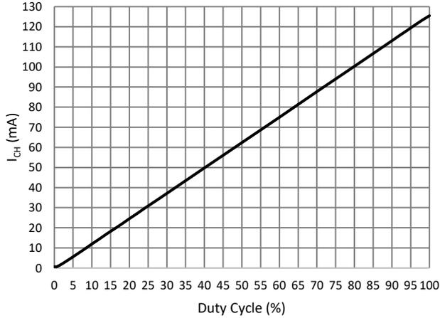
**PWM to Analog Dimming Curve @  $f_{PWMA} = 100\text{kHz}$**
