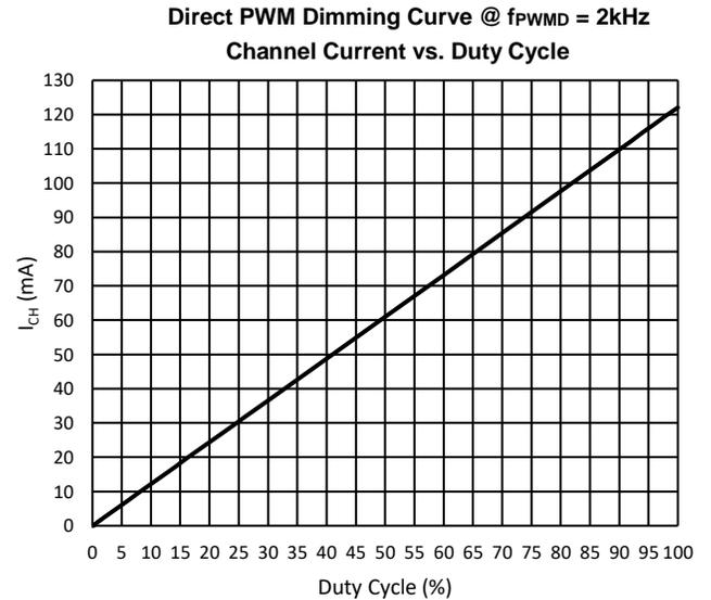
**Performance Characteristic** (continued) (@ $T_A = +25^\circ\text{C}$ ,  $V_{IN} = 20\text{V}$ ,  $V_{EN} = 5\text{V}$ , unless otherwise specified.)
