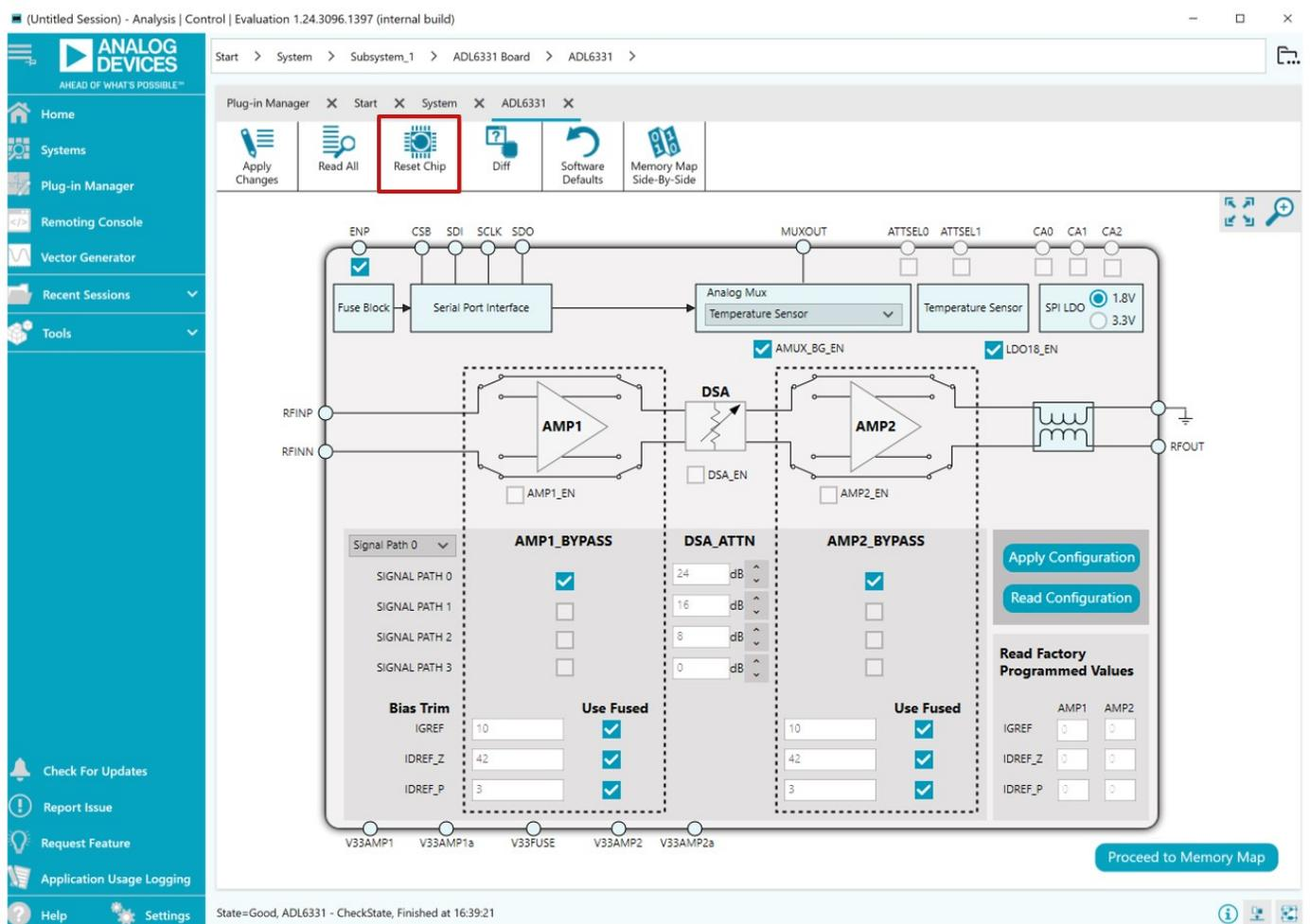
Figure 5. ADL6331-EVALZA Board Level View (After Reset Chip and ENP Set to High)
