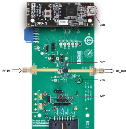
Figure 2. ADL6331-EVALZA and SDP-S Connections
