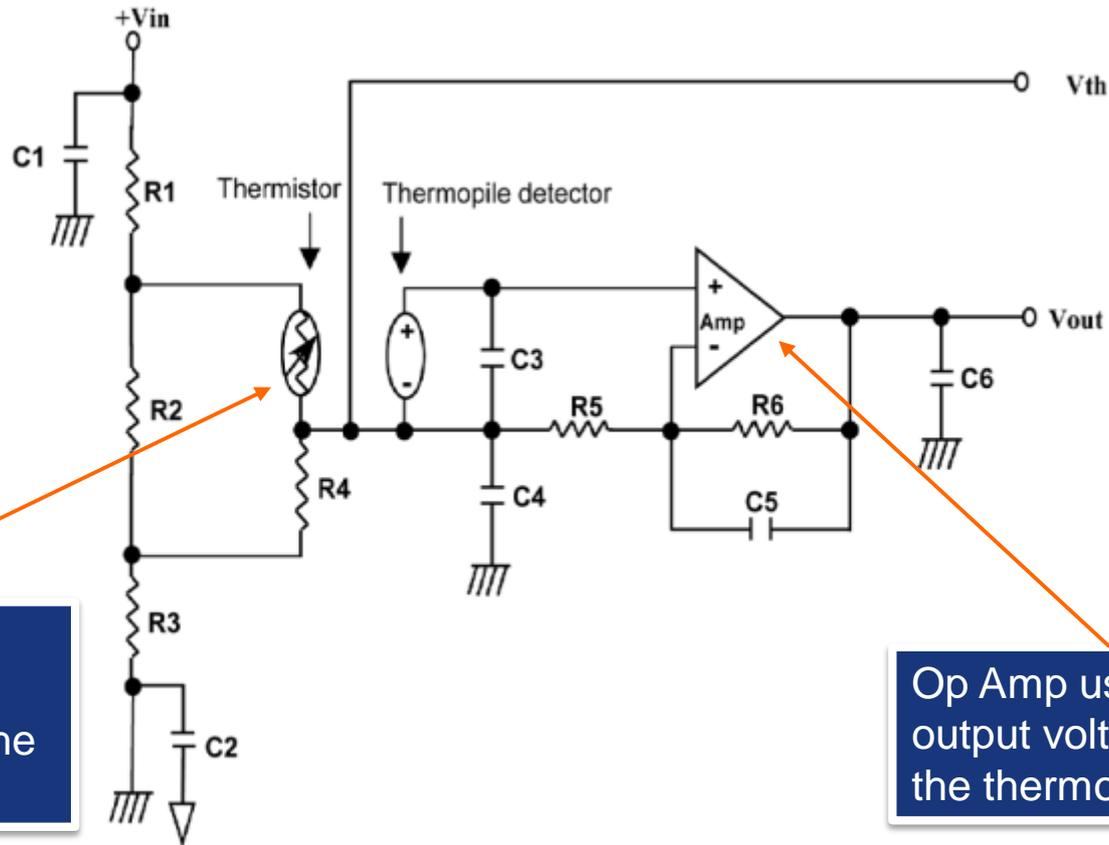
NTC Thermistor used for compensation of the ambient factors.
