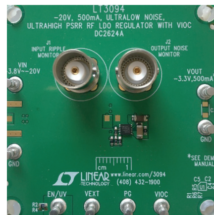
Figure 2. Demo circuit shows a tiny -3.3\ \text{V} solution.
