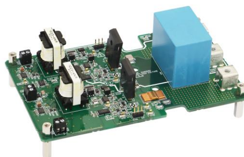
(b) 4 th generation SiC MOSFET EVK (Half-bridge)
