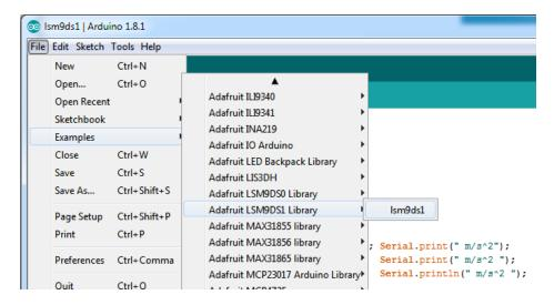
Then open up the Serial console at 115200 baud to read the sensor output! You'll get 9 distinct data points, accelerometer x/y/z in meters/s<sup>2</sup>, magetometer x/y/z in gauss and gyroscope in x/y/x degrees/second
