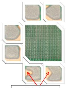
Crown and U shaped apertures have the greatest impact on midchip solder balling reduction. Phase two of the research evaluated four solder pastes that
