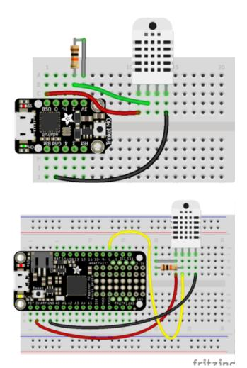
Here's an example using a Trinket MO you can use any CircuitPython board, just check that the Data pin is pulseiocapable.
