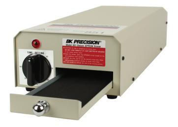
The model 851 is a heavy duty EPROM eraser that can simultaneously erase up to 40 twenty-four pin EPROM's. It is constructed of an all-metal case plus an advanced designed chip drawer that prevents UV radiation from being a hazard to the user. The chip drawer is lined with conductive foam to prevent electrostatic damage to the chips.
