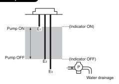
The pump starts when the water level reaches  $E_1$  (indicator ON) and stops when the water level drops below  $E_2$  (indicator OFF).
