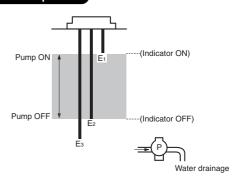
The pump starts when the water level reaches  $E_1$  (indicator ON) and stops when the water level drops below  $E_2$  (indicator OFF).
