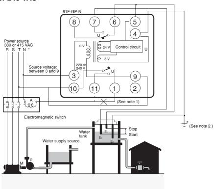
Note: 1. The diagram shows the connections for the water supply. When draining, change the connection from terminal 1 to terminal 11.
