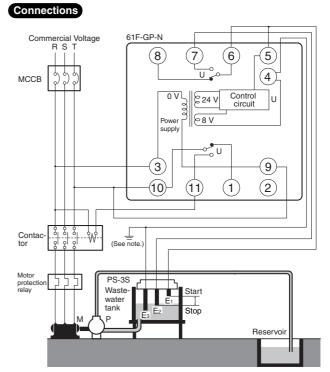
Note: Be sure to ground the common Electrode E3 (the longest Electrode).
