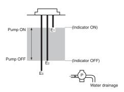
The pump starts when the water level reaches E<sub>1</sub> (indicator ON) and stops when the water level drops below E2 (indicator OFF).
