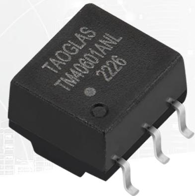
Featuring a compatible footprint with industry BMS Transformers, and designed to work in demanding automotive environmental conditions, the Taoglas TM40601ANL is a BMS Transformer with Common Mode Choke of 12 pins and Dual channel for Operation voltage of 1500VDC.
