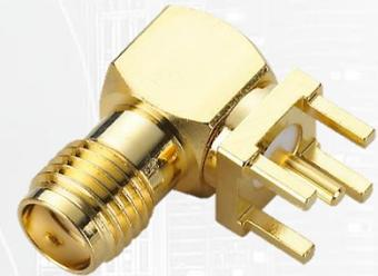
The PCB. SMAFRA.HT connector was designed to be mounted on a PCB. The maximum thickness of PCB that the connector can be used with is 0.4mm. The connector pin is directly soldered onto pads on the PCB. The connector is a standard SMA(F) RA Jack. Taoglas connectors are all RoHS compliant.
