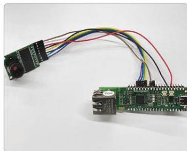
Integrates Arducam's 2MP module with a custom webserver on the W55RP20-EVB-Pico, enabling high-resolution image capture and chunk-based data delivery. Designed with robust buffer management, it smoothly handles large JPEG files—laying the groundwork for advanced camera features, dual-core operations, and potential live streaming extensions in future updates.
