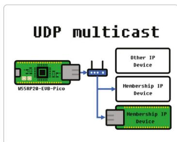
Explore an efficient data distribution method by broadcasting packets to multiple devices within the local network simultaneously.
