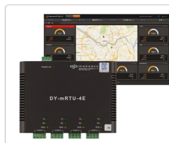
Powered by W55RP20, this solar power monitoring solution provides real-time energy tracking and remote diagnostics via Ethernet. By ensuring seamless data collection and analysis, it helps maximize efficiency in renewable energy installations—enabling smarter, data-driven decisions for sustainable power management.
