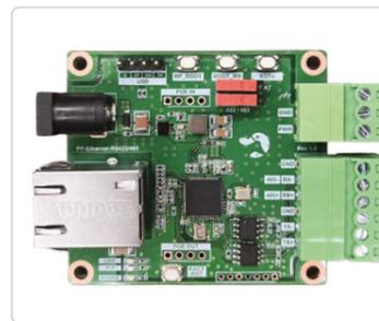
This industrial-grade RS485-to-Ethernet module, powered by WIZnet's W55RP20, ensures stable and low-latency communication in automation networks. Its robust design facilitates seamless data transmission between serial devices and Ethernet-based systems, making it an ideal solution for industrial IoT applications and remote monitoring setups.
