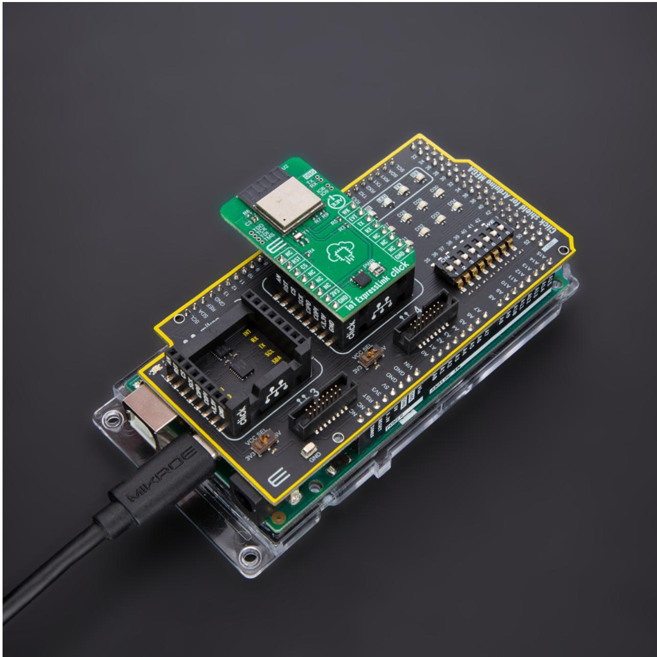
When the USB type C is connected to the Click Shield, the PWR diode will glow Blue, and at this setup, the connected Arduino Mega baseboard and all mikroBUS™ sockets will be powered from it.
