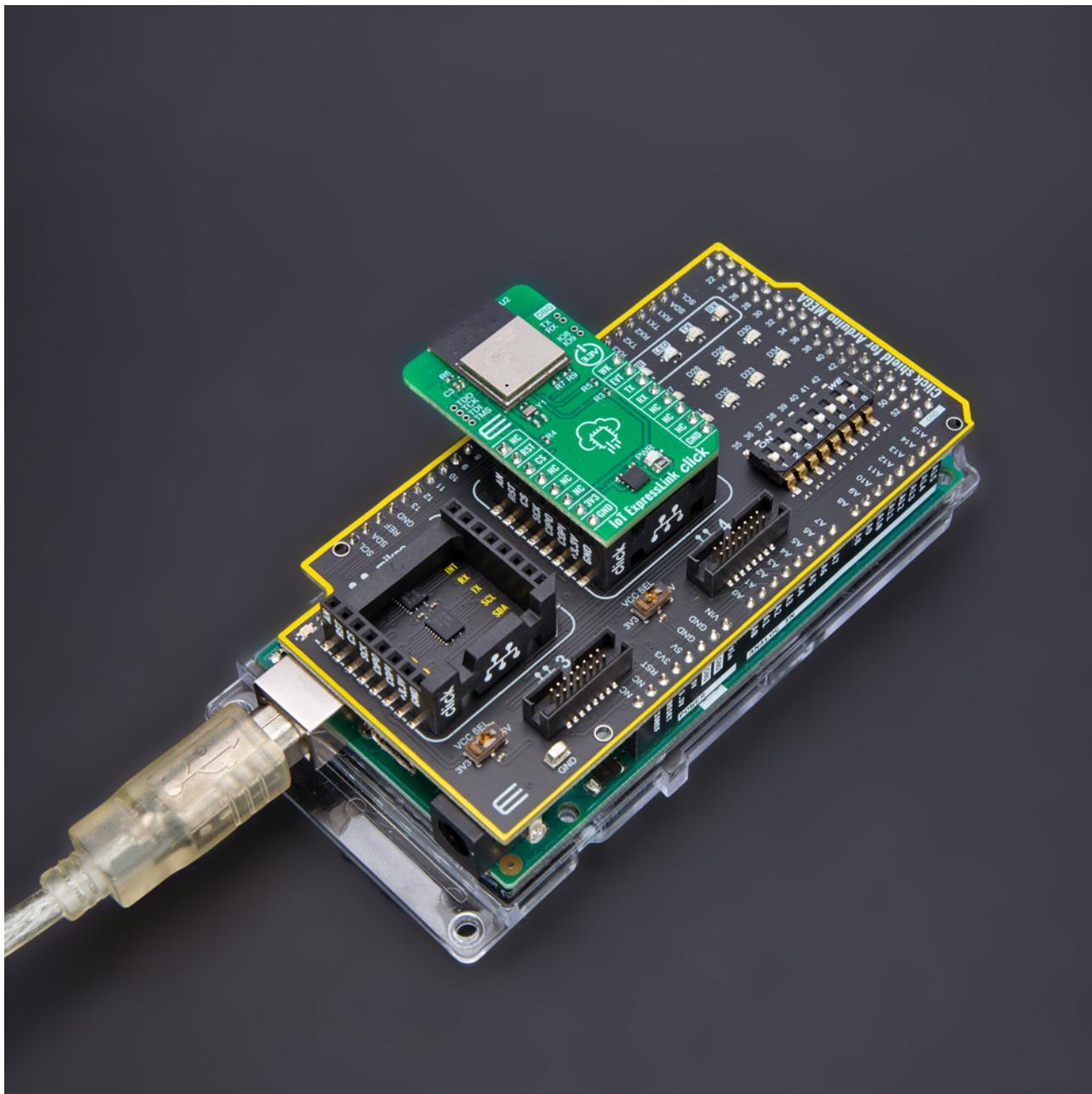
When the USB is connected to the Arduino Mega board, the PWR diode will glow Green, and at this setup, the Arduino Mega baseboard itself will be supplied, and it will provide power to the Click Shield, including all mikroBUS™ sockets.
