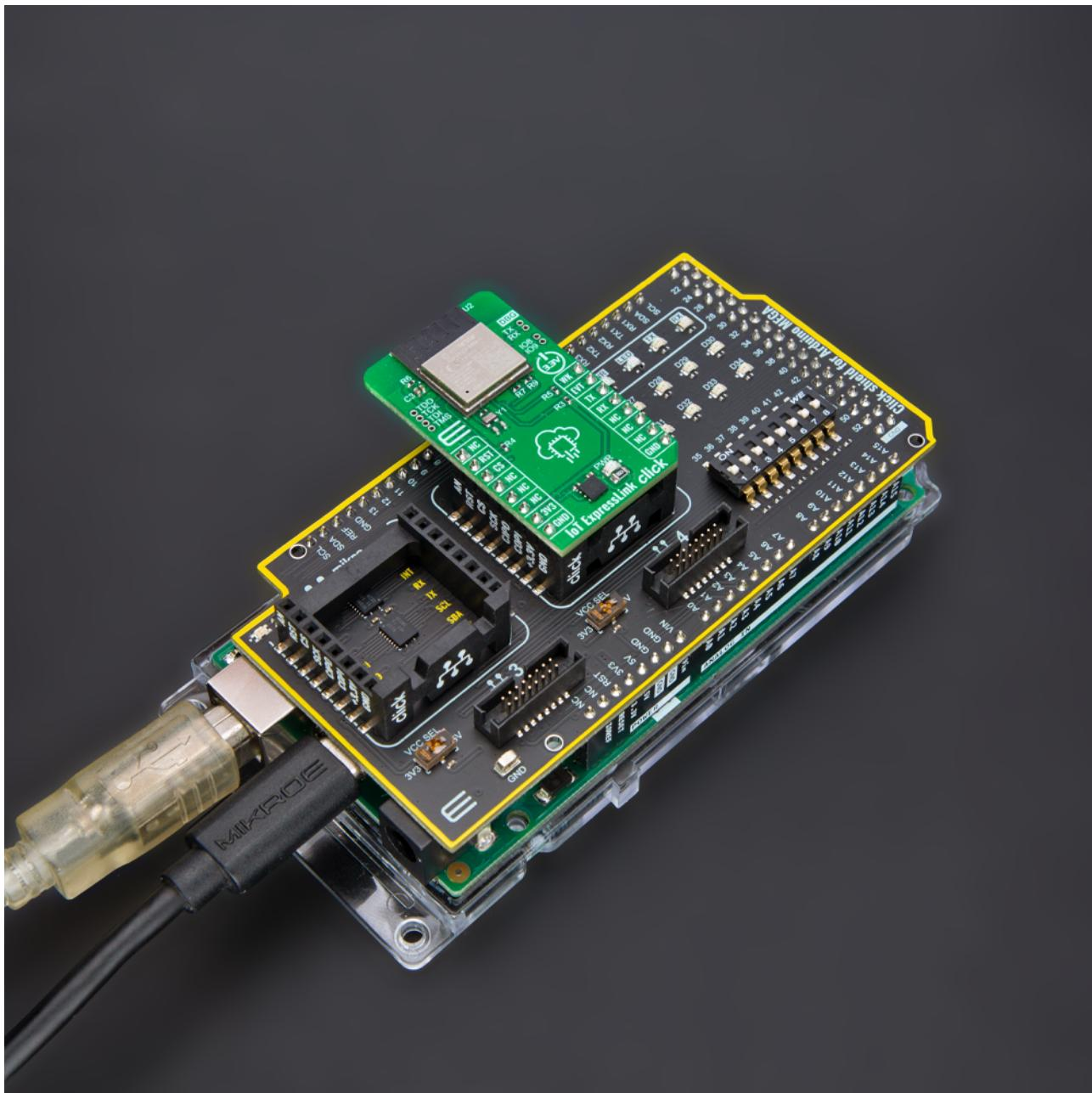
When the USB type C is connected to the Click Shield and the other USB is connected to the Arduino Mega board, the PWR diode will glow Cyan, and at this setup, the mikroBUS™ sockets are powered from the Click Shield.
