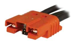
SBE® and SBO® connectors build on the capability of the two pole SB® connectors by offering up to 8 auxiliary power / signal contacts along with an IEC 60950 touch safe housing. The center of the main connector features a connector holder for either: two PP15/45, two PPMX, or APP's innovative 1x4 auxiliary connector.
