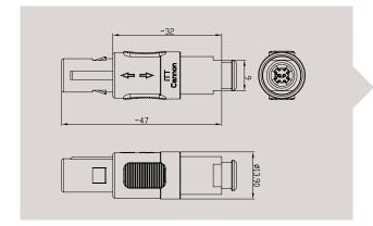
A3 Straight plug with cable collet and nut for bend relief
