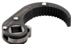
The Screwty® attachment is suitable for customisable M23 round plug-in connectors and for overmoulded M23 round plug-in connectors, with an outside dimension of the knurled nut of  $26.2 \pm 0.3$  mm. The tightening torque is 2-2.5 Nm.
