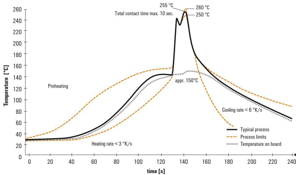
**Wave soldering profiles**
