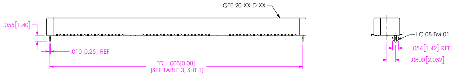
FIG 2 -LC: LOCKING CLIP OPTION (QTE-060-01-XXX-D-LC SHOWN) (DIFFERENT AS SHOWN, OTHERWISE SAME AS FIG 1)
