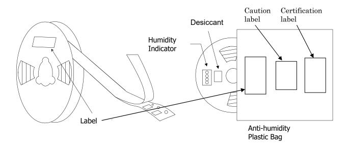
Tape and reel must be sealed with the anti-humidity plastic bag. The bag contains the desiccant and the humidity indicator.
