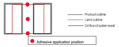
• Amount of adhesive applied is a standard 1/2 to 2/3 of the bottom flange thickness.
