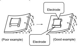
Products shall be located in the sideways direction (Length:a<b) to the mechanical stress.
