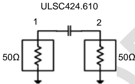
Figure 4 - 100nF ULSC measurement schematic
