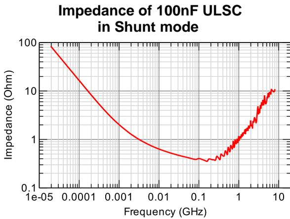
Figure 2 - 100nF ULSC Measured results (module of Z-parameters)
