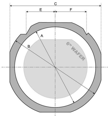
Figure 9 FF070 Frame with a 6" wafer
