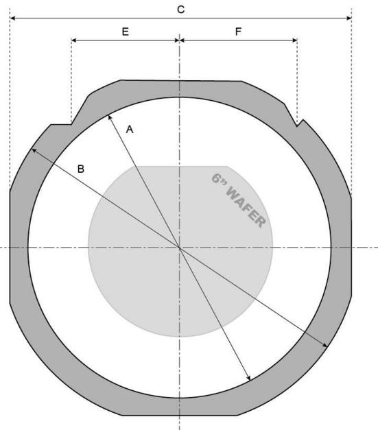
Figure 10 FF108 Frame with a 6" wafer
