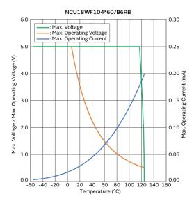
Max. Voltage, Max. Operating Voltage/Current Reduction Curve
