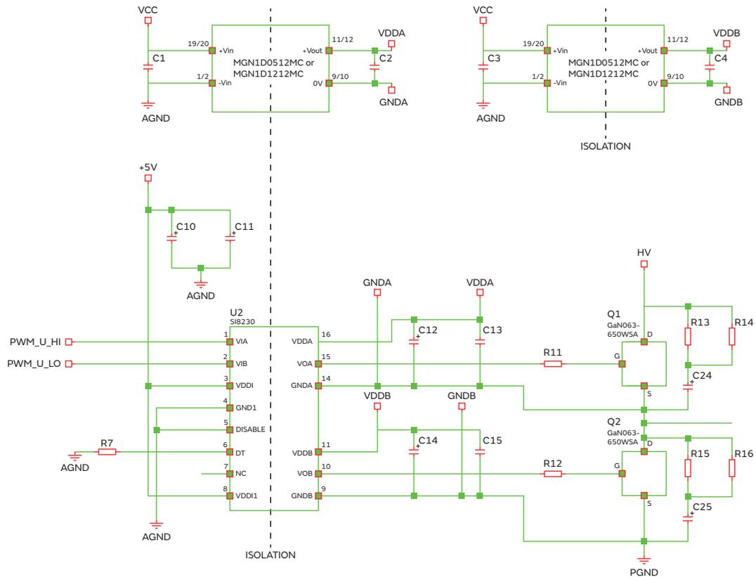
**Typical Application Circuit Diagrams - Navitas**
