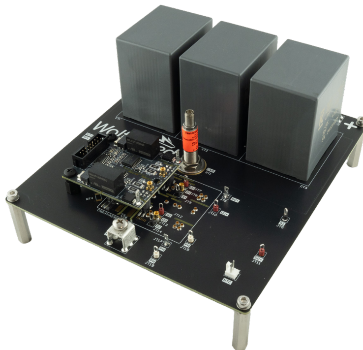
Figure 6: Example CGD1700HB2M-UNA attached to a power module evaluation board
