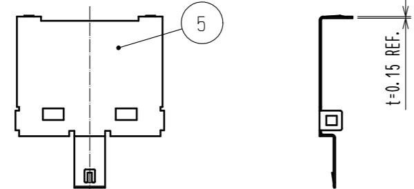
COVER CASE (A) WITH LOCK SPRINGS INSTALLED
