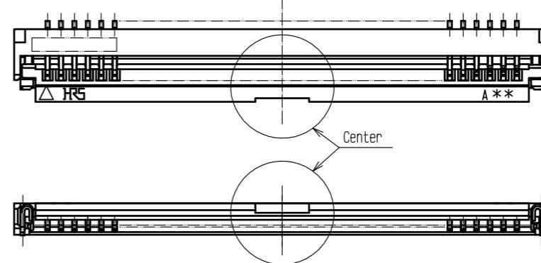
5. Do not pinch or pick the actuator to lift it as shown below. Otherwise, it may break.
