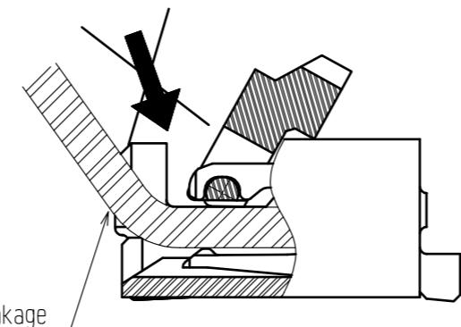
◆Checking the Locking Condition
