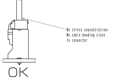
2) Since this product uses thick wires, a larger load is applied to the connector when inserting/extracting or routing the wires. Please use a retainer to reduce the load on the connector.
