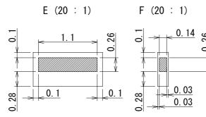
Connector lead on PAD layout ☐ PAD layout
