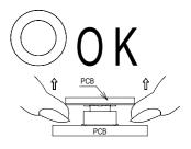
(2) When un-mating the connector, pull it out in parallel. If it is un-mated in an inclined position, connector may deform.
