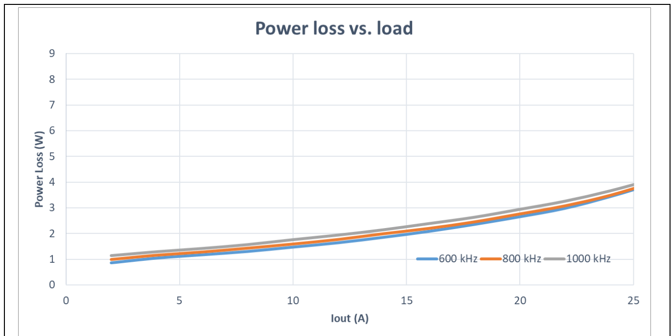
Figure 31 Power loss vs. load current without airflow in FCCM with external V_{CC} (12 V IN , 3.3 V OUT , no airflow, 470 nH, 800 kHz/1000 kHz, T a = 25°C)
