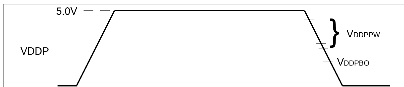
Figure 23 Supply Threshold Parameters
