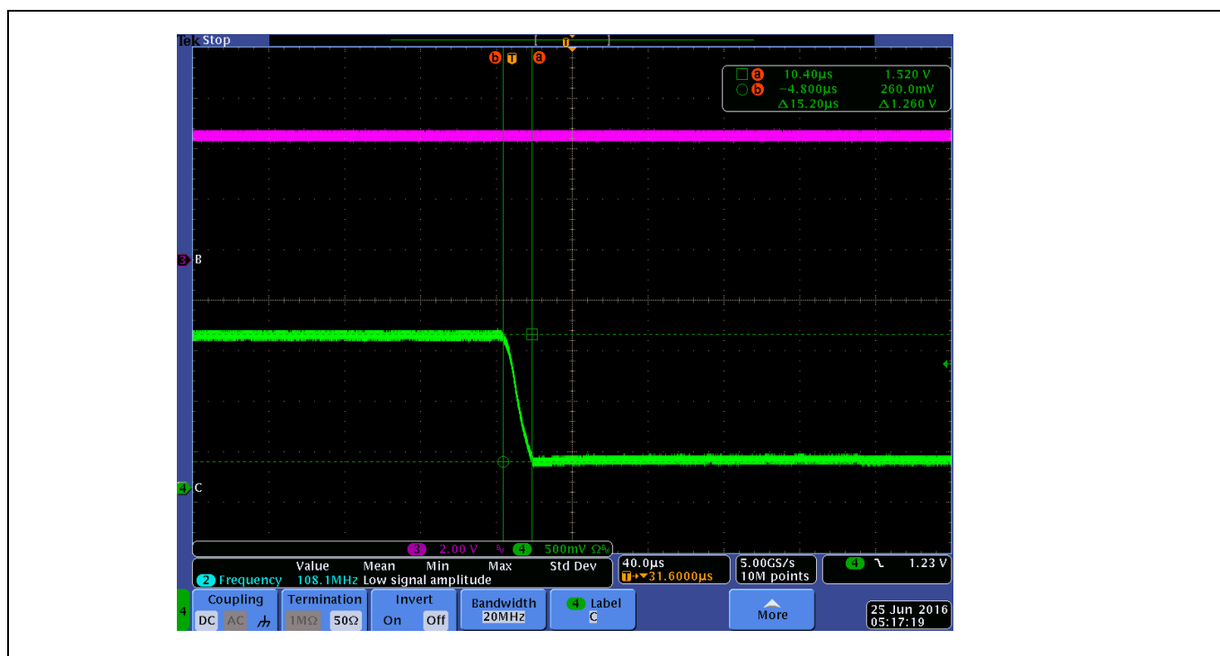
Figure 23 PINK=SM_ALERT#, GREEN=VOUT, After Enable is de-asserted, VOUT drops from 1.5 V to 0.27 V in 15 µs TOFF_FALL is 1 ms, Fixed_OVP_Thresh=1.35 V, VOUT=1.5 V
