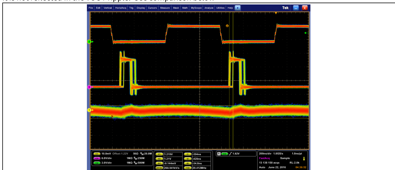
Figure 19 TOP→SYNC in, MIDDLE→SW_NODE, BOTTOM→RIPPLE
