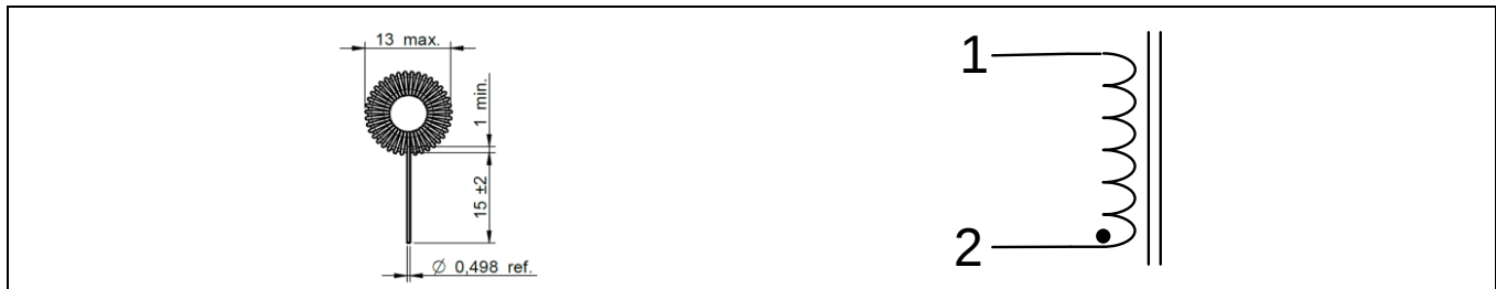
Figure 13 DM choke (side view) and electrical diagram
