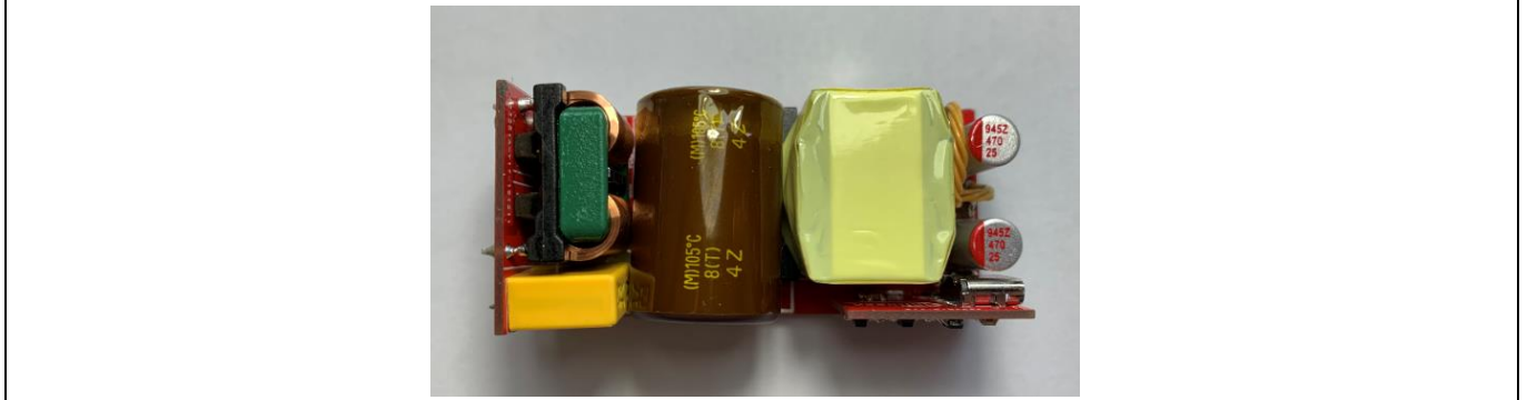
Figure 1 REF_XDPS21081_65W FQR ZVS flyback converter (top view)
