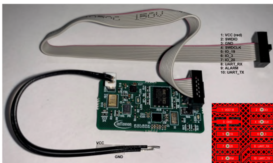
Figure 2 MicroIAS form-factor board connections
