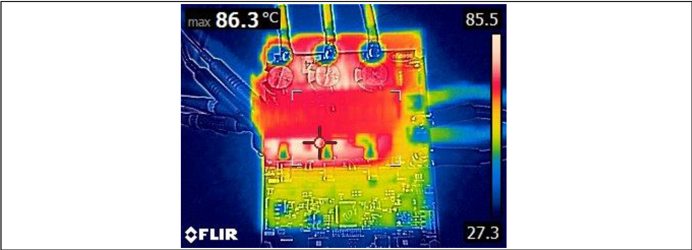
Figure 41 Thermal measurement, 86.3°C
