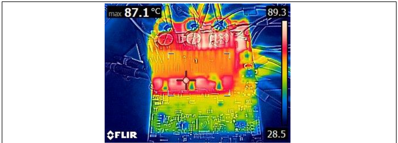
Figure 42 Thermal measurement, 87.1°C
