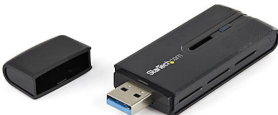
The USB867WAC22 USB 3.0 AC1200 Wireless Network Adapter lets you add Wireless-AC connectivity to a desktop or laptop computer through USB 3.0.
