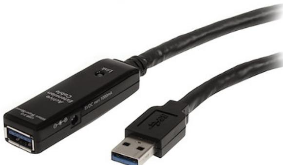
The USB3AAEXT5M, 5-meter Active USB 3.2 Gen 1 Extension Cable, offers one USB type-A (male) connector and one USB type-A (female) connector, and provides an active extension of USB 3.2 Gen 1 devices of up to 5-meters (16-feet).
