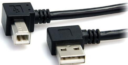
The USB2HAB2RA3 3ft USB A-to-B cable features a right angle USB 'A' male connector and a right angle USB 'B' male connector, for high quality connections to USB 2.0 peripherals such as USB printers, scanners or external USB hard drives, even in hard to reach areas and narrow spaces.
