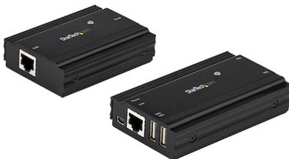
This USB 2.0 extender enables you to connect up to four USB 2.0 devices over distances of up to 330 feet (100 meters), over standard Cat5e/Cat6/Cat7 Ethernet LAN cabling.
