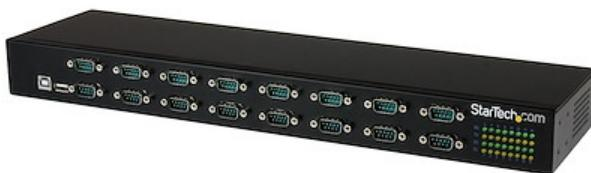
Here's an easy and cost-efficient way to add RS232 serial capability to your industrial setting. This 16-port USB-to-serial adapter hub features a sturdy, rack-mountable chassis, and supports daisy chaining, so you can connect multiple hubs together to increase your serial device port count.
