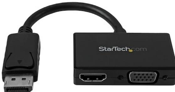
This DisplayPort to HDMI + VGA travel adapter lets you connect your DP enabled Ultrabook or laptop computer to any VGA or HDMI display.
