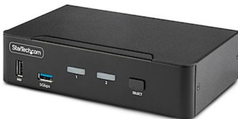
Share and switch between two USB-A and DisplayPort-enabled computers, using this DisplayPort KVM Switch. Share an 8K 60Hz DisplayPort monitor, a keyboard and mouse, two USB 5Gbps devices, and two additional USB 2.0 devices.
