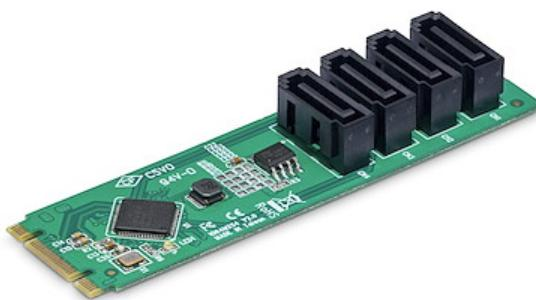
Add up to four independent SATA drives to a desktop via a single 2280 M.2 drive slot, maintaining SATA 6Gbps read/write speeds per drive.
