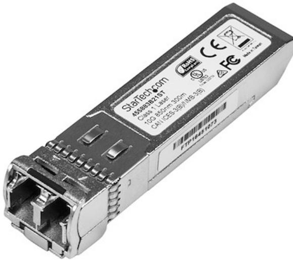
The 455883B21ST is a TAA compliant HPE 455883-B21 compatible fiber transceiver module that has been designed, programmed and tested to work with HPE brand switches and routers. It delivers dependable 10 GbE connectivity over fiber cable, for 10GBASE-SR compliant networks, with a maximum distance of up to 300 m (984 ft).
