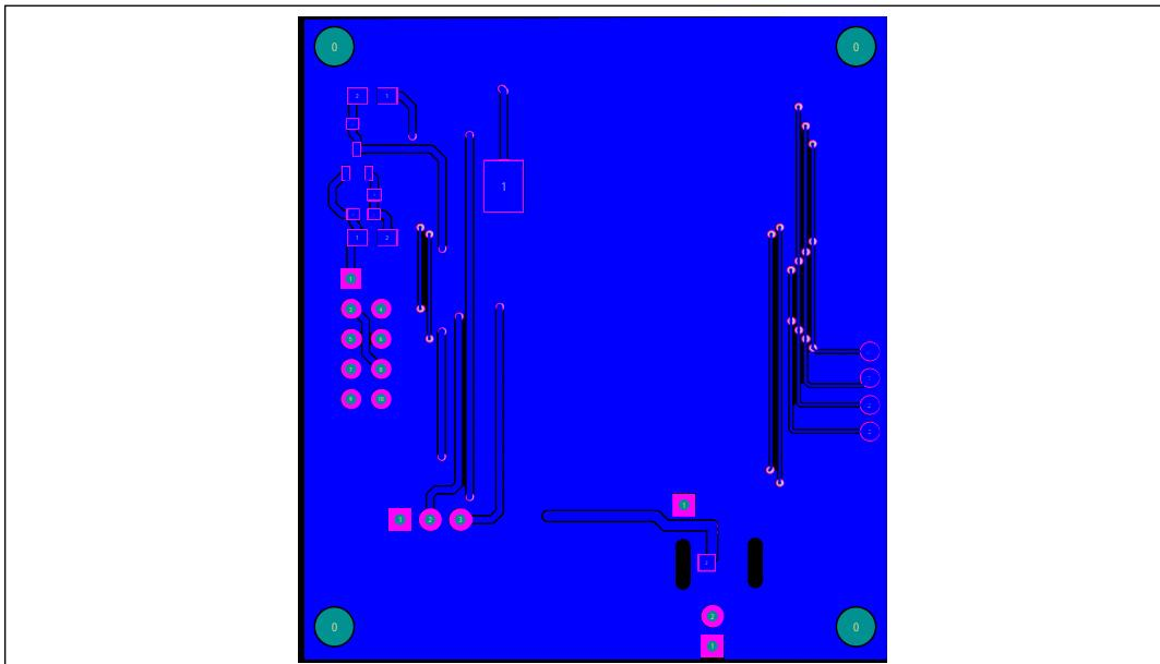
**Figure 9** Board PCB Layout - Bottom Layer
