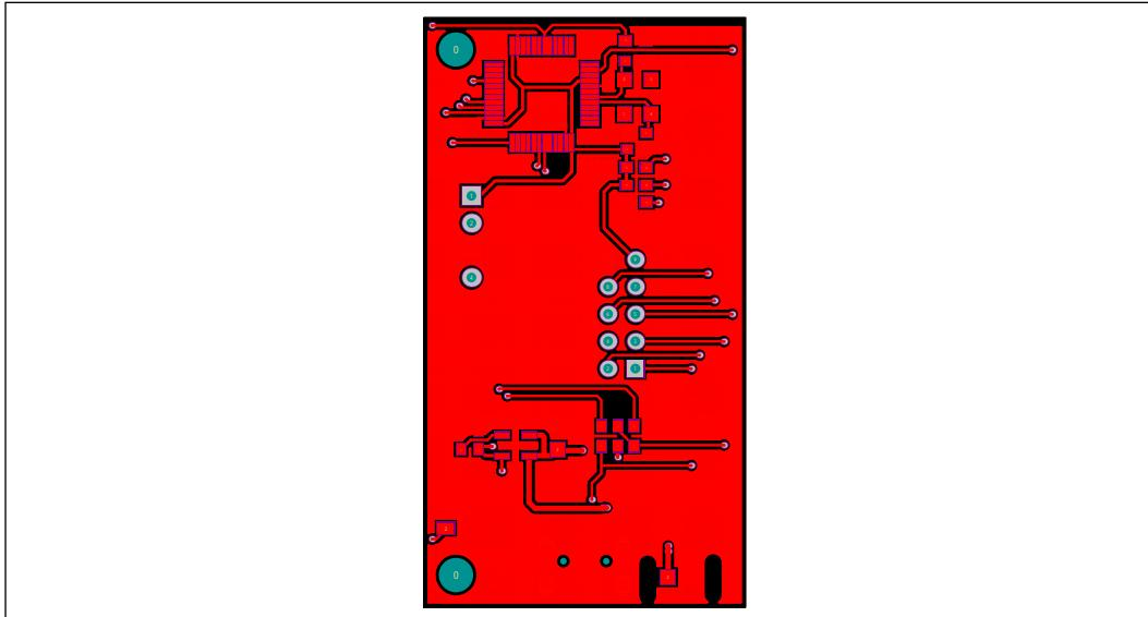
Figure 11 Board PCB Layout - Top Layer
