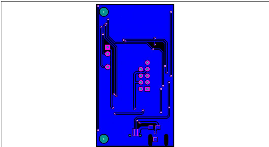
Figure 13 Board PCB Layout - Bottom Layer
