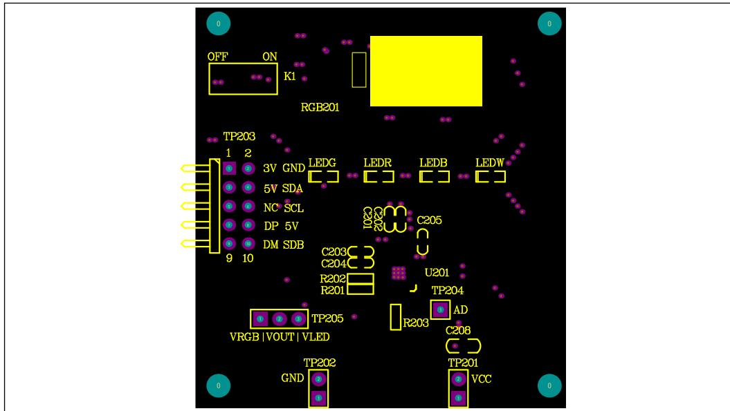
Figure 6 Board Component Placement Guide - Top Layer
