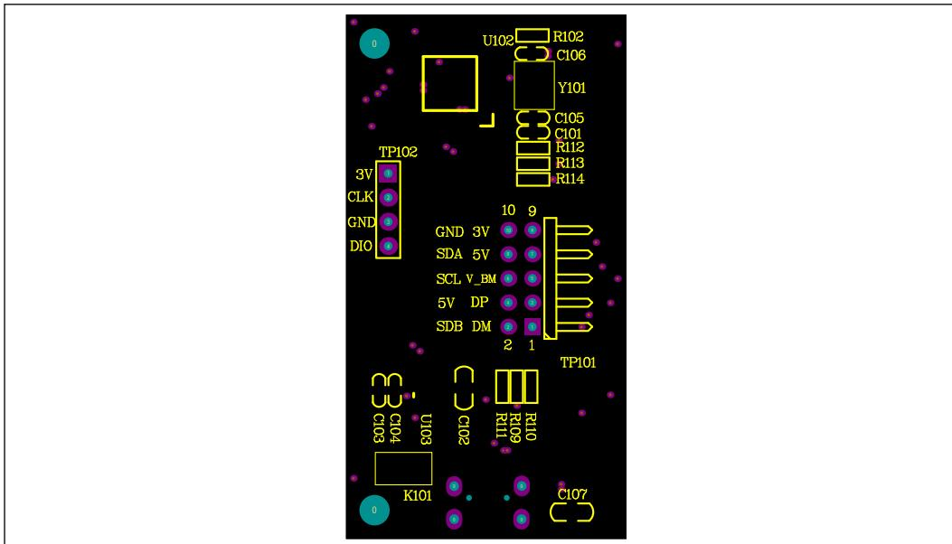
Figure 10 Board Component Placement Guide - Top Layer
