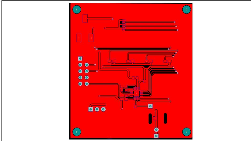
Figure 7 Board PCB Layout - Top Layer
