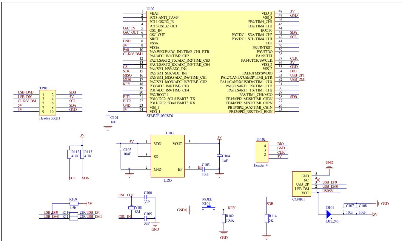
Figure 5 MCU Board Schematic
