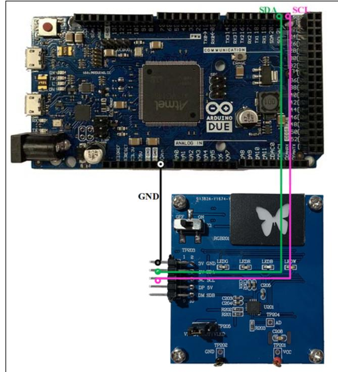
Figure 3 Arduino DUE connect to RGBW Board
