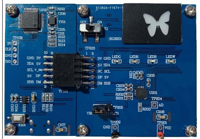
Figure 1 Photo of IS31FL3197-QFLS2 Evaluation Board
