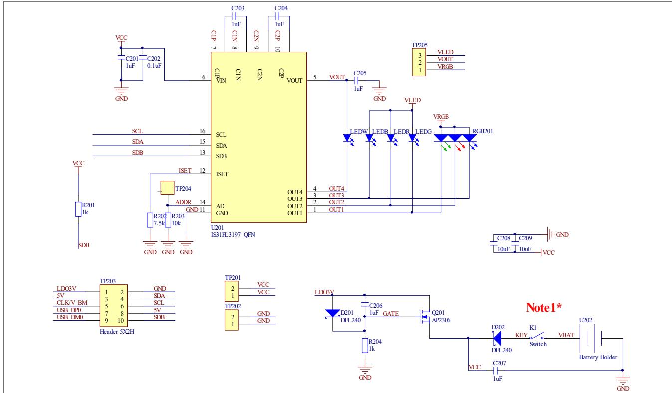
Figure 4 IS31FL3197 RGBW Board Schematic
