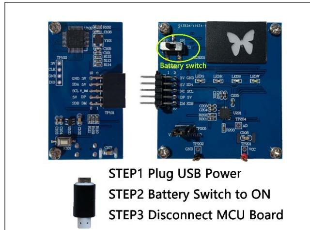
Figure 2 RGBW Board disconnect from MCU board
