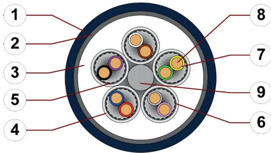
1. Outer jacket: Pressure extruded, halogen-free TPE mixture
