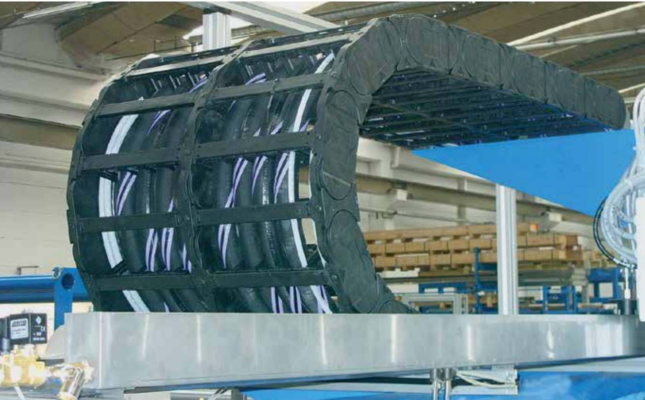
E4-1 as a noise-optimized version with extension links. Unsupported application with high fill weight. Assembled with rigid hydraulic hoses. The max. noise level can be reduced up to 9dB(A) using the optional rubber dampers
